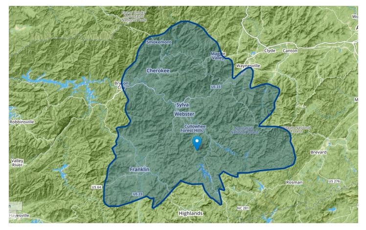
Due to the unique mountainous terrain, not all radios will receive a "city grade" signal in all locations as indicated on the map above. The map is a computer projection and approximates the actual "city grade" coverage of 95.3 WWCU FM.
